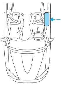
The side air bags are fitted on the outboard side of the seatbacks of the front seats. In certain lateral collisions, the air bag on the side affected by the collision will be inflated, even if the respective seat is not occupied. The air bag was designed to inflate between the door panel and occupant to further enhance the protection provided occupants in side impact collisions.
